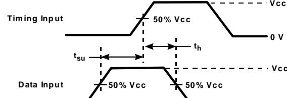
VOLTAGE WAVEFORMS SETUP AND HOLD TIMES
