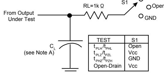
LOAD CIRCUIT FOR 3-STATE AND OPEN-DRAIN OUTPUTS
