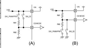
Intermediate voltage can be generated by RM1 and RM2. Please set the value of each R1, R2, RM1, RM2 at around 100k . For switches, CPU open-drain I/O port and transistor can be used.
