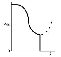
Fig.17 Vds waveform at turn on (with adequate R5)
