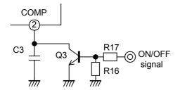
Fig.34 ON/OFF control circuit (1)
