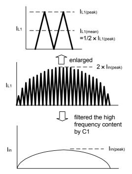
Fig.3 Outline of inductor and AC input current
