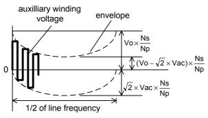
Fig.14 Auxiliary winding voltage
