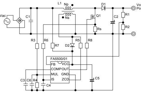
Fig.13 Typical application circuit
