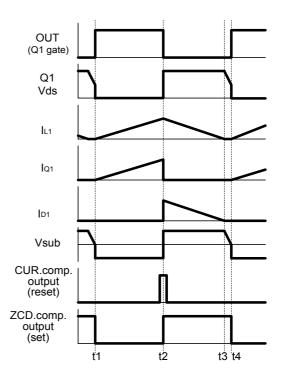
Fig.2 Timing chart of switching operation
