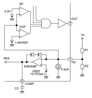
Fig.5 Error amplifier circuit
