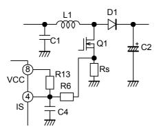
Fig.32 Compensation circuit of surge current
