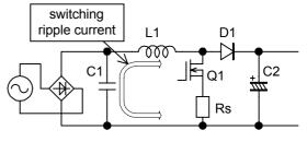
Fig.27 Input capacitor circuit
