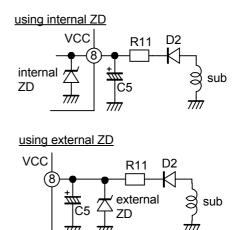
Fig.15 Vcc clamp circuit
