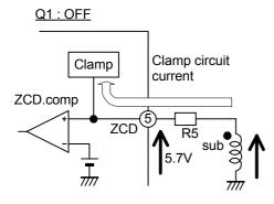
Fig.11 Clamp circuit of ZCD pin(2)
