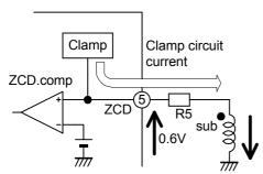
Fig.10 Clamp circuit of ZCD pin(1)
