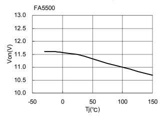
UVLO startup threshold(Von) vs. junction temperature(Tj)
