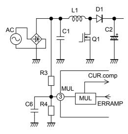
Fig.7 Multiplier circuit
