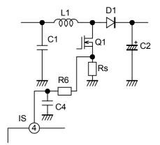
Fig.24 IS pin circuit
