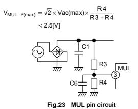
In an actual circuit, the rectified voltage contains many noises from switching. To avoid this influence, a capacitor C6 is typically connected between MUL pin and GND pin. If the capacity of C6 is too small, the filtering is not effective. If the capacity is too large, the input voltage of MUL pin is distorted and then AC input current is also distorted. In calculating, the cutoff frequencies determined with C6 and R3, R4 should be
