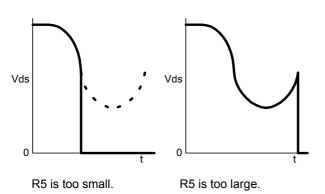
Fig.18 Vds waveform at turn on
