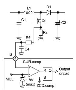
Fig.8 Current sense comparator circuit
