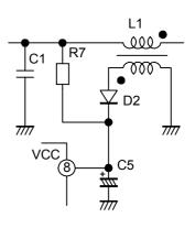
Fig.19 Vcc pin circuit
