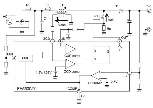
Fig.1 Outline of PFC converter circuit
