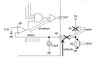
Fig.6 Open/short protection at FB pin
