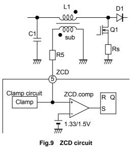
A resistor for current limit is typically connected between the ZCD pin and the auxiliary winding because of rating current of ZCD pin. While MOSFET is on, negative voltage is generated in the auxiliary
