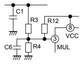
Fig.30 Compensation circuit of dead time
