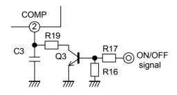
Fig.35 ON/OFF control circuit (2)
