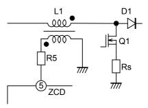
Fig.16 ZCD pin circuit
