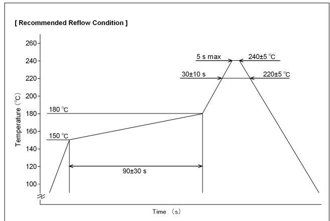
$\mbox{\%}$  Max 2 cycles of the above reflow profile should be applied.
