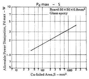
\* The measured values of Pd represent the values measured when solder on the Cu-foiled area is all wet.
