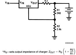
Use of  $\mathrm{R}_{\mathrm{S}}$  allows low charging rates with fully charged battery.
