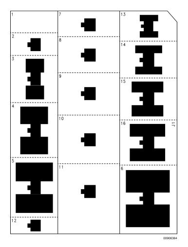
FIGURE 12. Top View of the Thermal Test Pattern in Actual Scale
