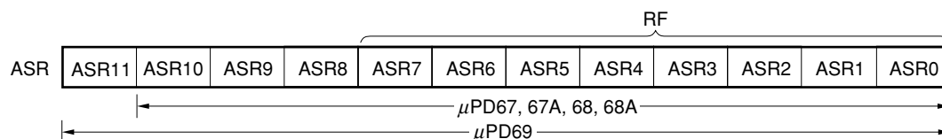
Figure 2-2. Address Stack Register Configuration
