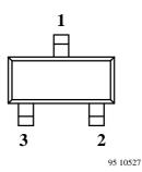
S869TR Marking: 69R Plastic case (SOT 23) 1= Collector; 2= Base; 3= Emitter
