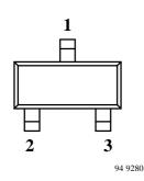
S869T Marking: 869 Plastic case (SOT 23) 1= Collector; 2= Base; 3= Emitter
