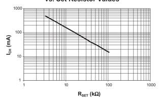
Operating Supply Current vs. R<sub>SET</sub> (V<sub>IN</sub> = 5V)
