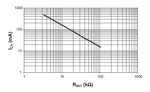
Figure 2: Constant Charging Current vs. Set Resistor Values.
