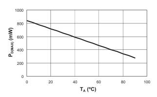
Figure 3: Maximum Power Dissipation.
