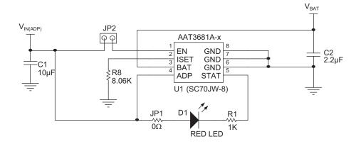
Figure 7: AAT3681A Evaluation Board Schematic Diagram.
