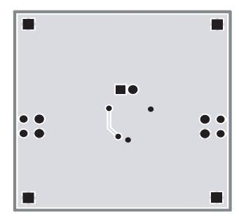
Figure 6: AAT3681A Evaluation Board Bottom Side Layout.
