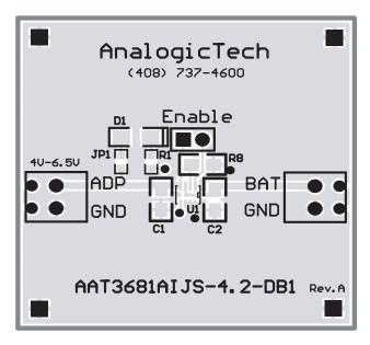
Figure 5: AAT3681A Evaluation Board Top Side Layout.
