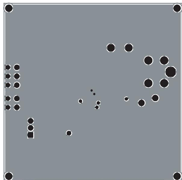
Figure 5: AAT3687 Evaluation Board Solder Side Layout.
