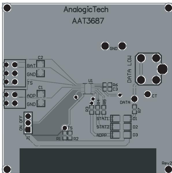
Figure 4: AAT3687 Evaluation Board Component Side Layout.
