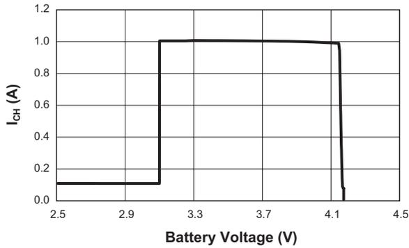
**Fast Charge Current vs. Supply Voltage**
