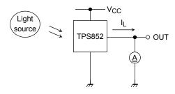
Note 5: Switching time measurement method
