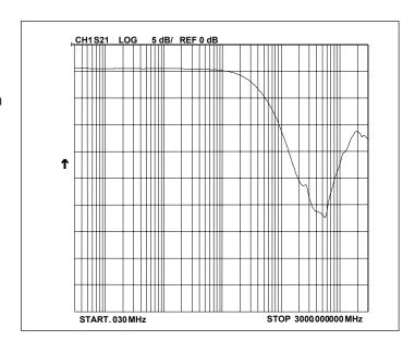
Figure 2 - Typical Insertion Loss S21
