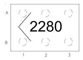
3 x 2 Grid Flip Chip TVS (Top View)
