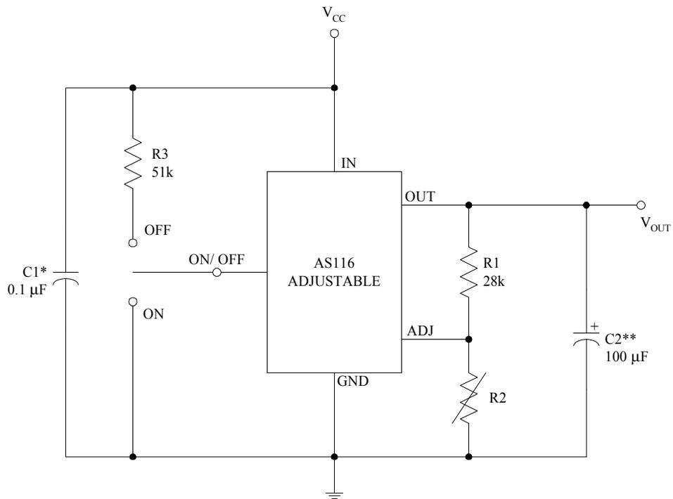
$$V_{OUT} = \text{Reference Voltage} \times \frac{R1 + R2}{R1}$$
