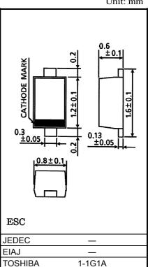
Mounted on a glass epoxy circuit board of 20 × 20 mm, pad dimension of 4 × 4 mm.
