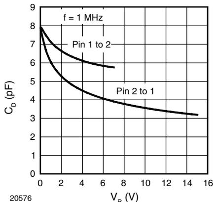
Figure 3. Typical Capacitance  $C_D$  vs. Reverse Voltage  $V_R$
