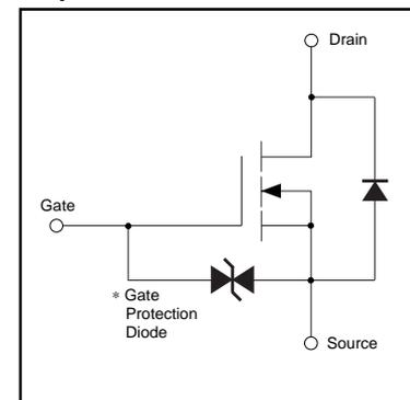
\*A protection diode is included between the gate and the source terminals to protect the diode against static electricity when the product is in use. Use a protection circuit when the fixed voltages are exceeded.
