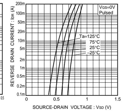
Fig.9 Reverse drain current vs. source-drain voltage (I)
