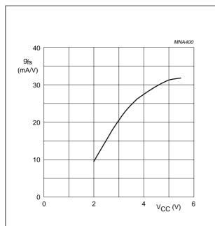
Fig.11 Typical forward transconductance  $g_{fs}$  as a function of the supply voltage at  $T_{amb} = 25 \, ^{\circ}\text{C}$ .
