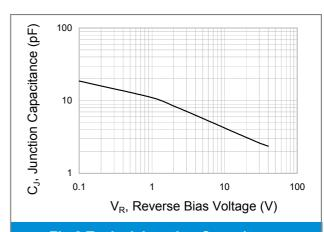
Fig.2 Typical Junction Capacitance
