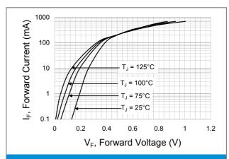
Fig.4 Typical Forward Characteristics
