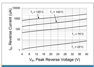
Fig.3 Typical Reverse Characteristics
