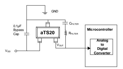
Figure 5. Digital Temperature output through a microcontroller
