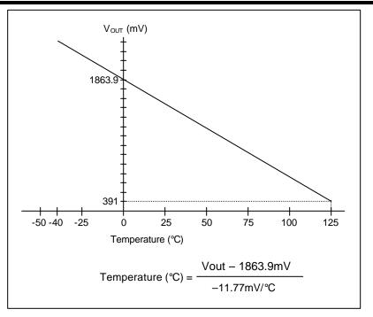
Figure 1. aTS20 Output Voltage vs. Temperature
