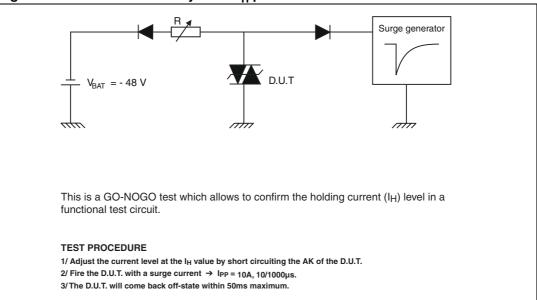
Figure 17. Test circuit 3 for dynamic I<sub>H</sub> parameter
