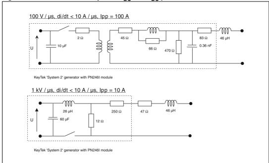
Figure 15. Test circuit 1 for Dynamic  $\rm I_{BO}$  and  $\rm V_{BO}$  parameters
