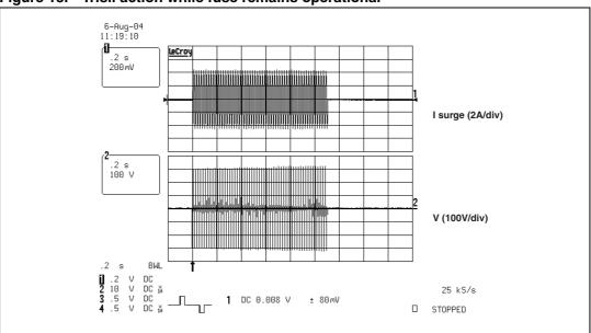
Figure 13. Trisil action while fuse remains operational
