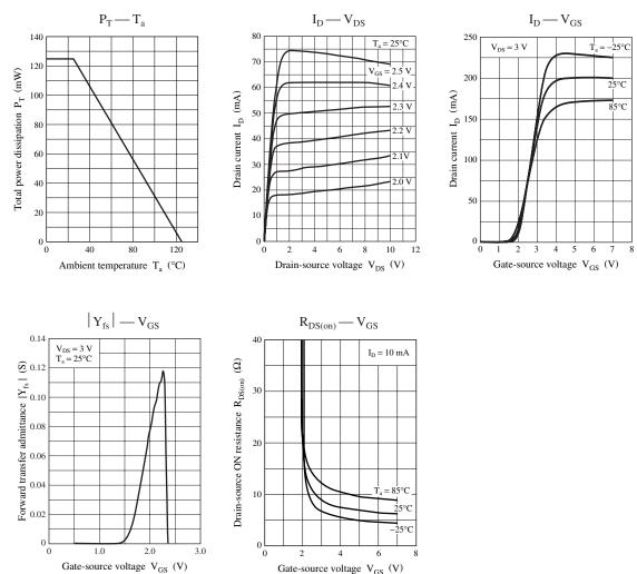
Gate-source voltage V<sub>GS</sub> (V)
