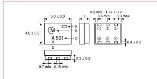
(Thickness: T is mentioned on character table) Description Code Code Description Mark of Input Terminal С Delay Time (nominal value) Α В Symbol Marking D Impedance Code
