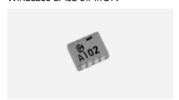
This delay line has been developed by utilizing advanced multilayer technology. It is comprised of a copper line and temperature compensated dielectric NPO (0  $\pm$  60ppm/°C) and includes a metal shield. This results in a very small device that is compatible with high frequency applications and SMD chip processing.
