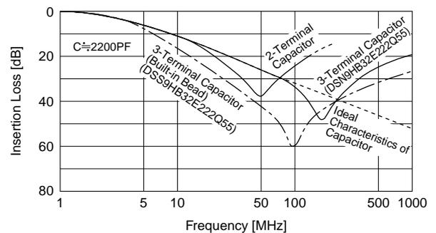
A 3-terminal capacitor has a higher self resonance frequency than a general 2-terminal type and exhibits effective noise suppression at high frequency.
