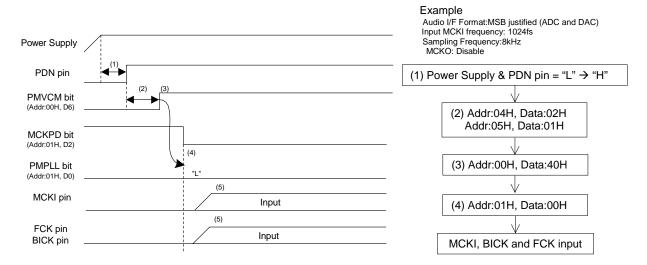
Figure 46. Clock Set Up Sequence (4)
