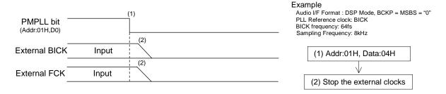
Figure 53. Clock Stopping Sequence (2)
