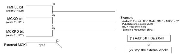
Figure 54. Clock Stopping Sequence (3)
