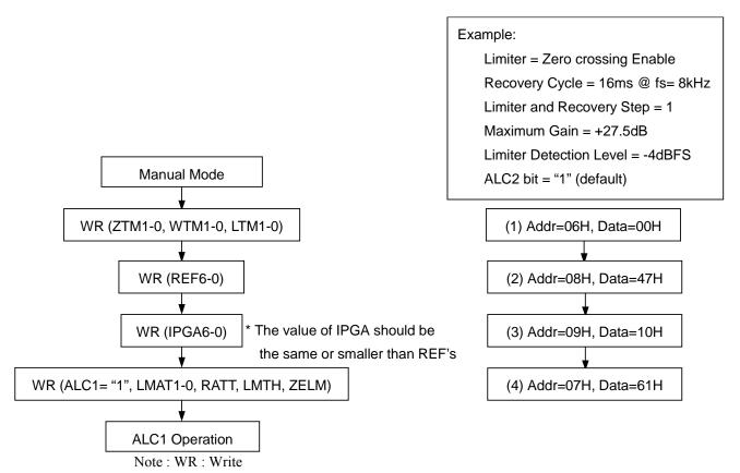
Figure 30. Registers set-up sequence at the ALC1 operation
