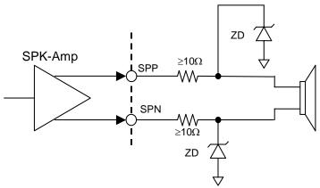
Figure 34. Circuit of Speaker Output(Load Capacitance > 30pF)
