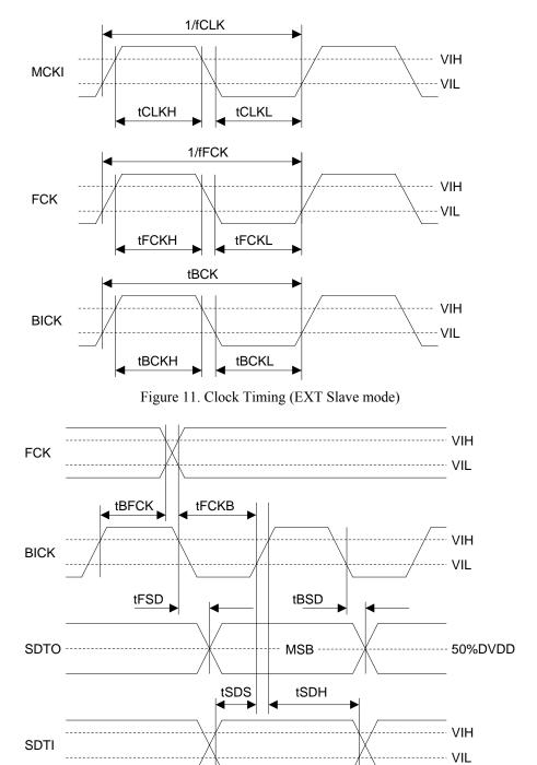
Figure 12. Audio Interface Timing (PLL, EXT Slave mode & Except DSP mode)
