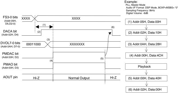
Figure 50. Mono Lineout Sequence
