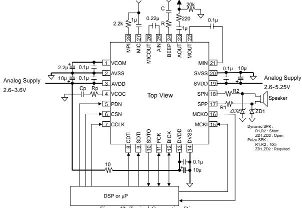
Figure 42. Typical Connection Diagram
