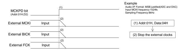
Figure 55. Clock Stopping Sequence (4)
