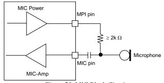
Figure 29. MIC Block Circuit
