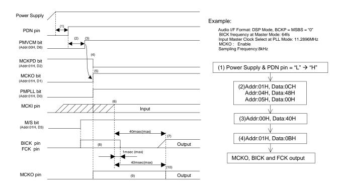
Figure 43. Clock Set Up Sequence (1)
