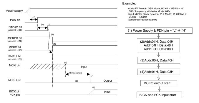
Figure 45. Clock Set Up Sequence (3)
