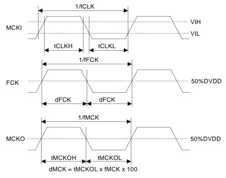
Figure 2. Clock Timing (PLL Master mode)
