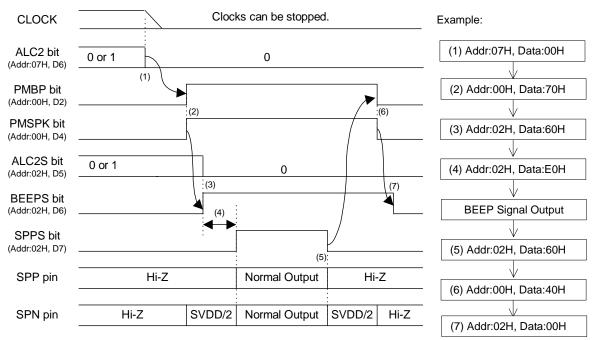
Figure 49. "BEPP-Amp → Speaker-Amp" Output Sequence
