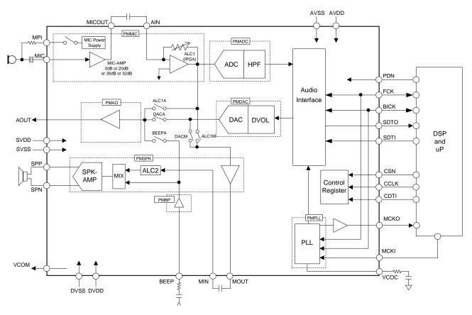
Figure 1. AK4631 Block Diagram
