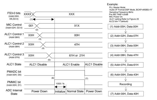
Figure 47. MIC Input Recording Sequence
