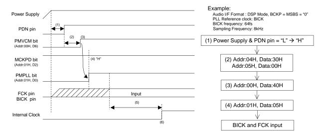
Figure 44. Clock Set Up Sequence (2)
