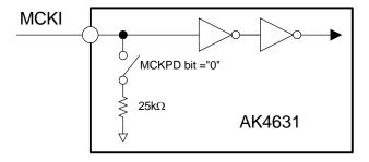
Figure 17. Pull-down resistor of MCKI pin
