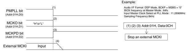
Figure 52. Clock Stopping Sequence (1)
