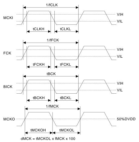
Figure 8. Clock Timing (PLL Slave mode; PLL Reference Clock = MCKI pin & Except DSP mode)
