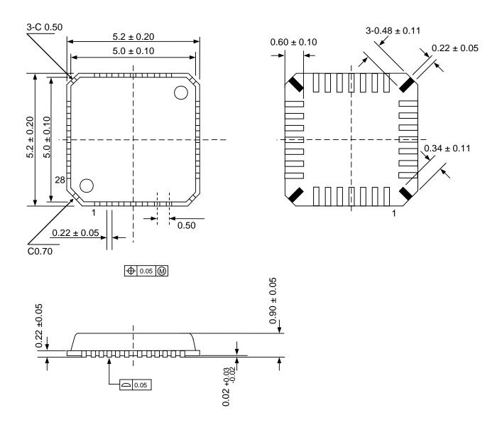
Note) The part of black at four corners on reverse side must not be soldered and must be open.
