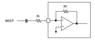
Figure 31. Block Diagram of BEEP pin
