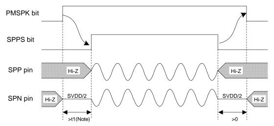
Figure 35. Power-up/Power-down Timing for Speaker-Amp
