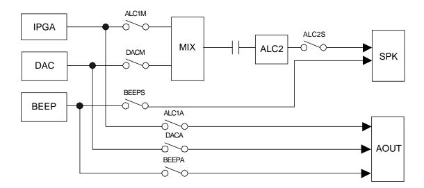
Figure 41. Speaker and Mono Lineout-Amps switch control
