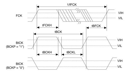
Figure 7. Clock Timing (PLL Slave mode; PLL Reference Clock = FCK or BICK pin & DSP mode; MSBS bit = "1")
