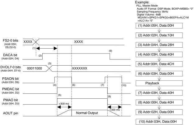
Figure 51. Mono Lineout Sequence
