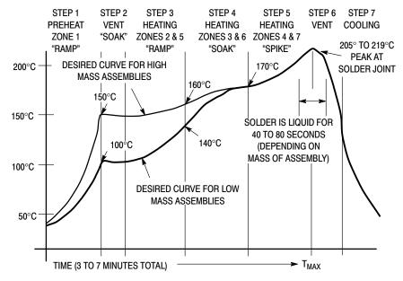
Figure 1. Typical Solder Heating Profile
