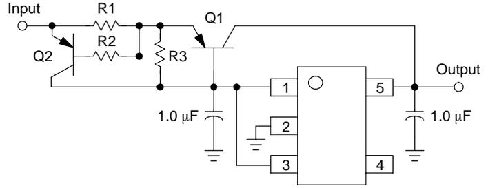
**Figure 15. Current Boost Regulator with Short Circuit Limit**
