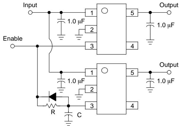
**Figure 16. Delayed Turn-on**
