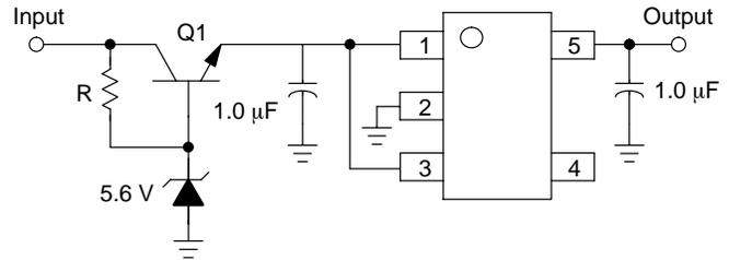
**Figure 17. Input Voltages Greater than 6.0 V**
