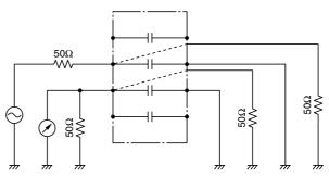
Measurement were performed by wiring this product onto a printed circuit board configured as in the diagram above.
