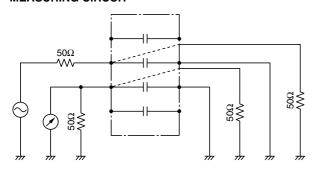
Measurement were performed by wiring this product onto a printed circuit board configured as in the diagram above.
