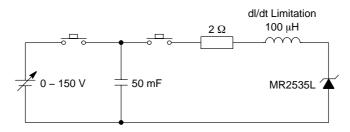
Figure 12. Load Dump Test Circuit
