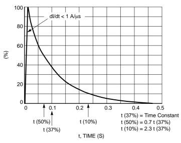
Figure 13. Load Dump Pulse Current
