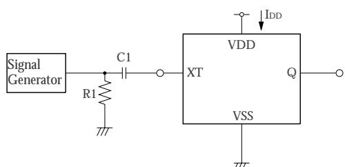
2.0V<sub>P-P</sub>, 30MHz sine wave input signal (3V operation)
