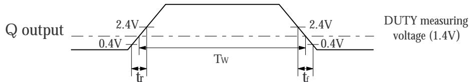
**Output duty cycle (CMOS)**
