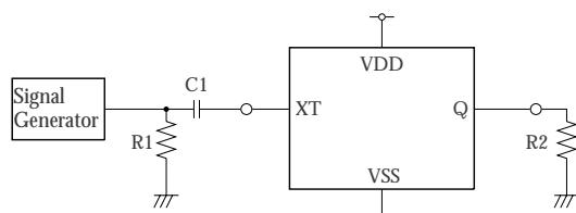
2.0V<sub>P-P</sub>, 10MHz sine wave input signal (3V operation)
