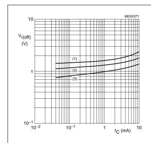
TR1 (NPN);  $V_{CE} = 5 \text{ V}.$
