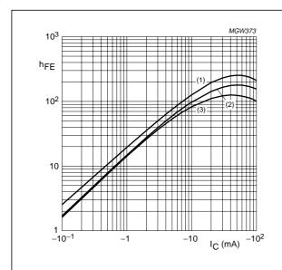
TR2 (PNP);  $V_{CE} = -5 \text{ V}.$
