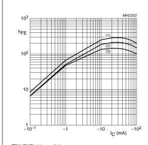
TR2 (PNP);  $V_{CE} = -5 \text{ V}.$
