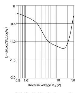
Fig.4 Linearity factor Vs. Reverse voltage
