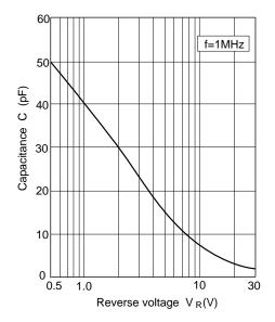
Fig.2 Capacitance Vs. Reverse voltage
