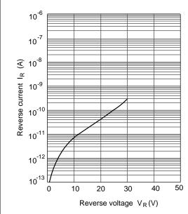
Fig.1 Reverse current Vs. Reverse voltage
