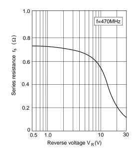
Fig.3 Series resistance Vs. Reverse voltage
