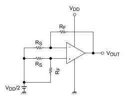
SVRR  $V_{DD} = 1.8 \text{ V}: V_{DD} = V_{DD}1, V_{OUT} = V_{OUT}1$  $V_{DD} = 7.0 \text{ V}: V_{DD} = V_{DD}2, V_{OUT} = V_{OUT}2$
