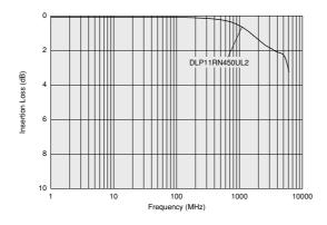
■ Differential Mode Transmission Characteristics (Typ.) **DLP11RB Series**
