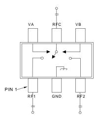
DC blocking capacitors not required if negative control voltage is used.
