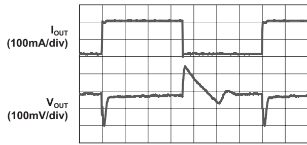
LDOB Load Transient Response
